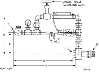
\*Between flange proportioner is standard. Upon request, proportioners can also be supplied in flanged style. Note: In-line balanced pressure proportioners require a minimum of 5 pipe diameters of straight, unobstructed water inlet supply pipe.
