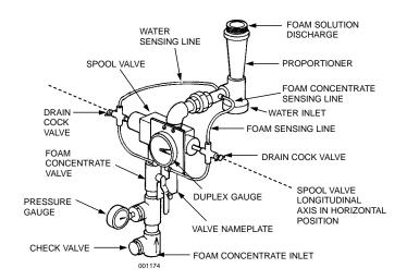
$\ensuremath{\textbf{Note:}}$  Spool valve must be installed with the longitudinal axis in the horizontal (level) position.
